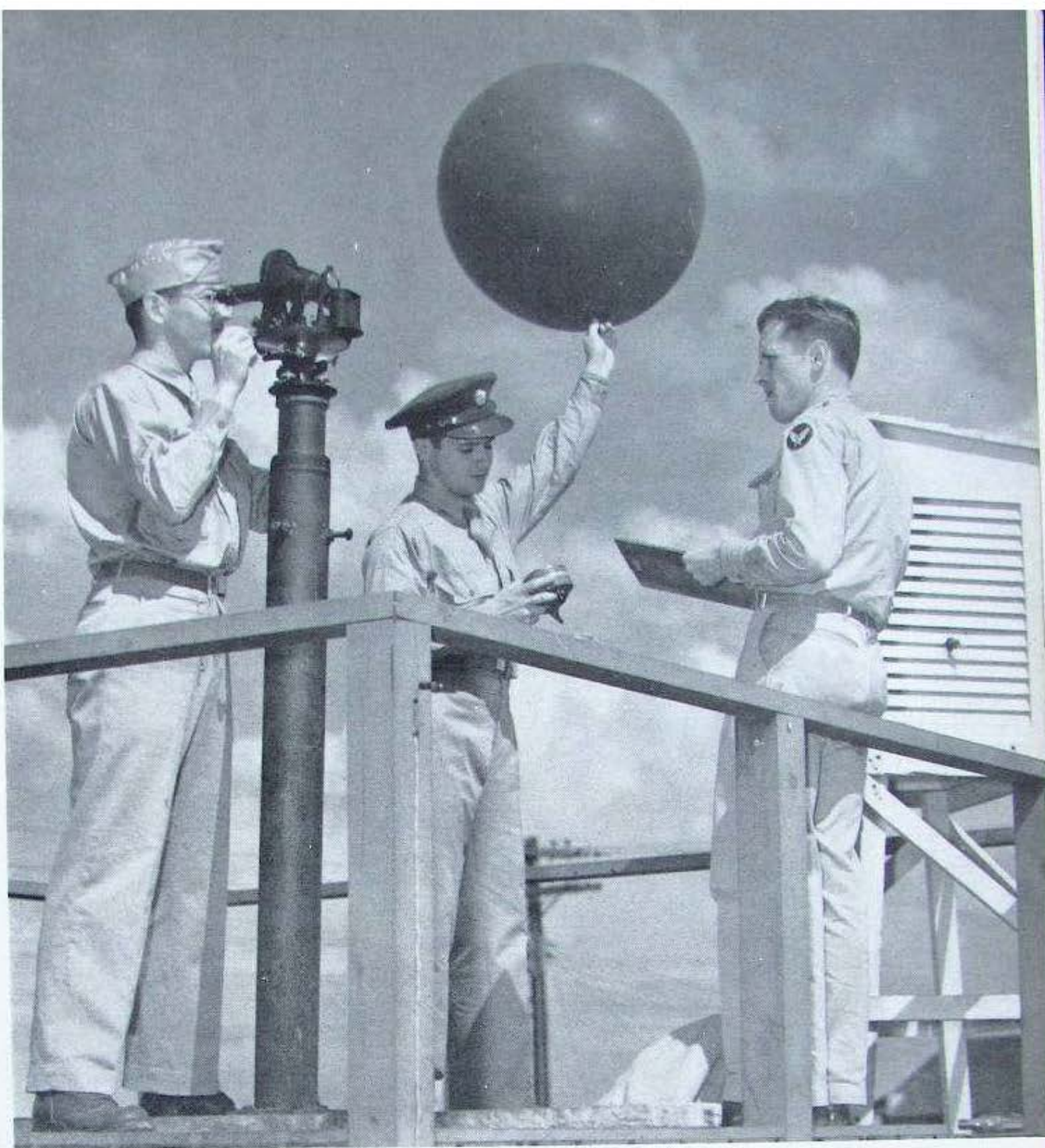
Aerologists send up a hydrogen-filled balloon to plot wind aloft. Balloon is checked with theodolite.
