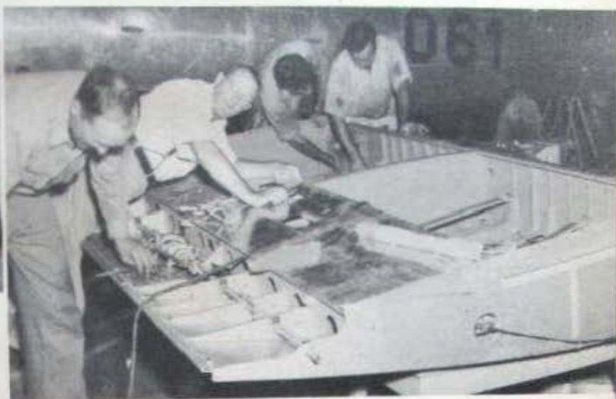
Ample facilities are at hand for rebuilding damaged parts, such as this wing section.
