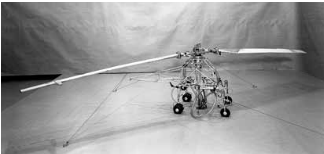
A 13-foot-diameter, dynamically scaled, tip-driven rotor was used to power this 1/10 -scale model of the Hughes XH-17 for investigations of flutter characteristics. The model was tested in the west return passage of the Full-Scale Tunnel. (NACA LAL 66021)
