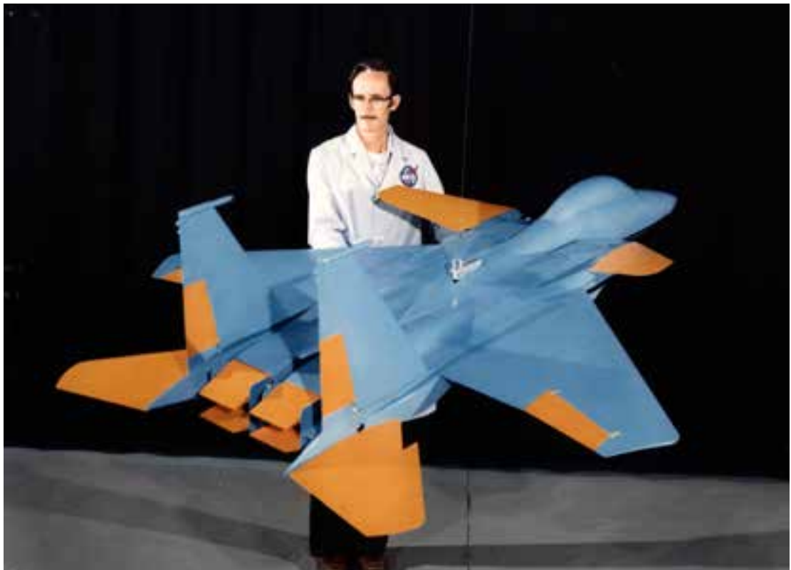
Technician Dave Robelen poses with the free-flight model of the F-15 STOL/MTD aircraft prior to free-flight testing in 1985. (NASA L-85-7469)
