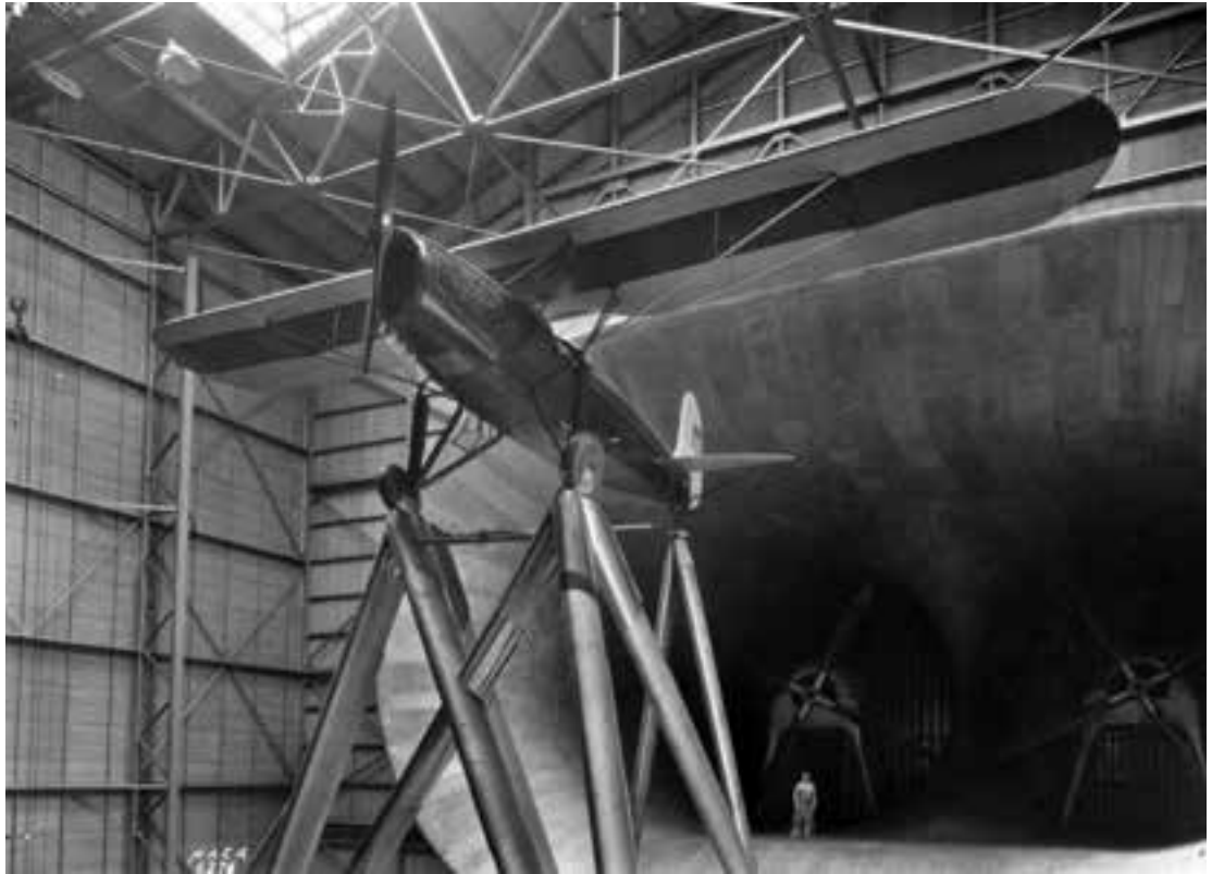
The first Fairchild F-22 research aircraft procured by the NACA was tested to determine its lift and drag characteristics in 1932. Note the early NACA badge emblem on the vertical tail indicating NACA ownership of the aircraft. (NACA 6276)
