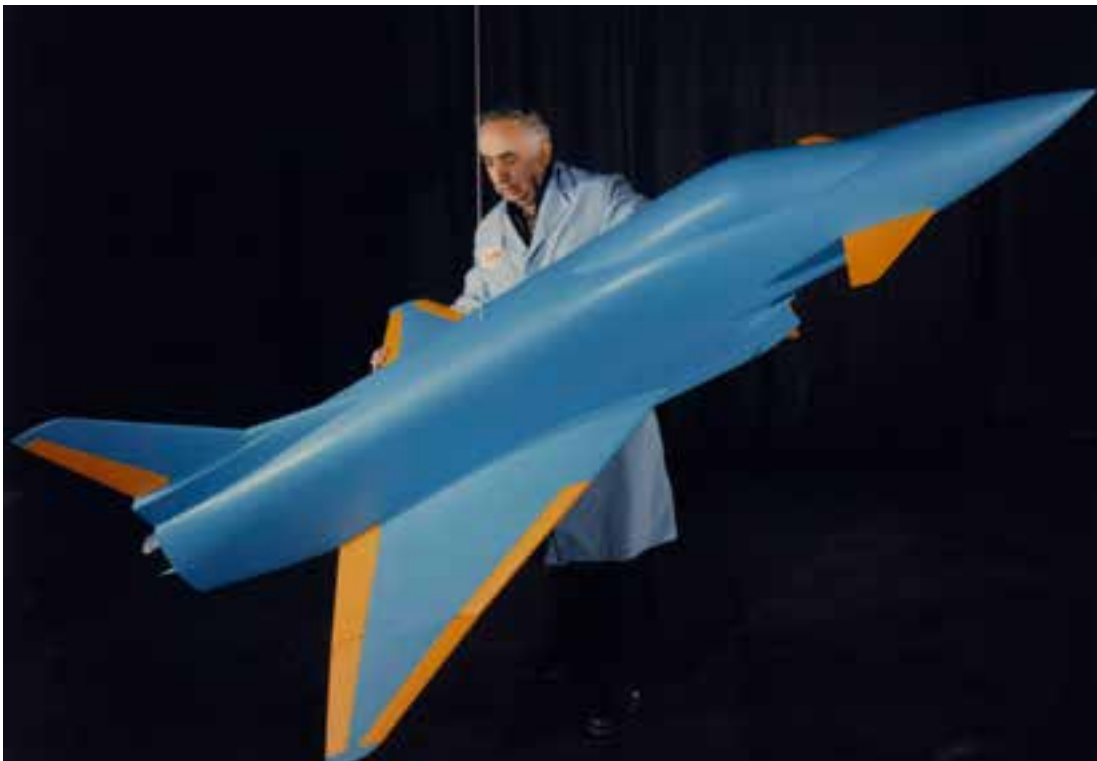
An early version of the X-31 configuration is readied for free-flight tests in 1988. The staff of the Full-Scale Tunnel was a major contributor to the success of the research project and provided rapid-response solutions to problems that were encountered during aircraft flight tests at Dryden. (NASA L-88-13225)
