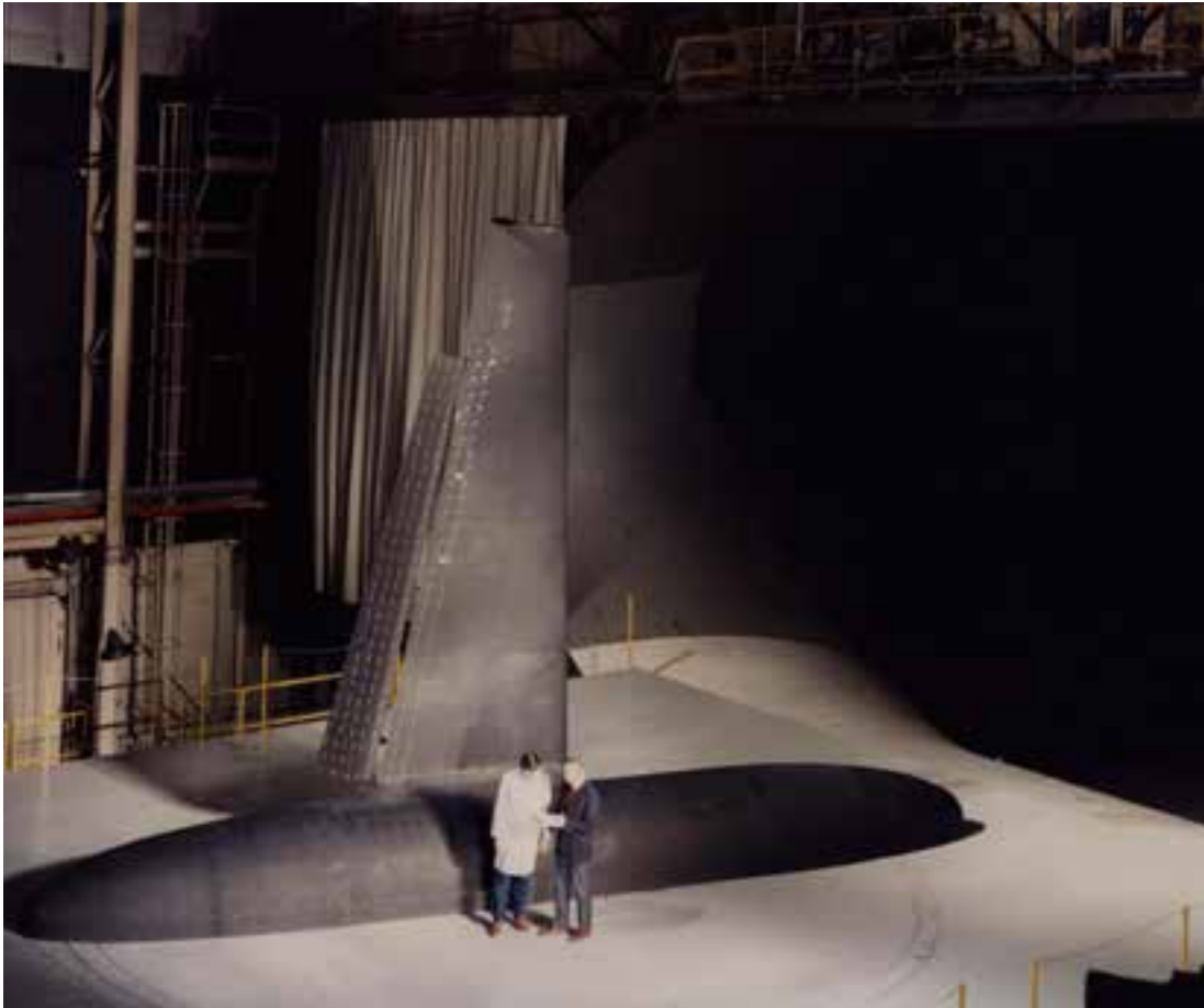
Frank Jordan (right) confers with technician Jim Staples during tests of a full-scale semispan model of the Peregrine wing in the Full-Scale Tunnel in 1987. Note the wool tufts attached to the wing and trailing-edge flap for flow-visualization studies. (NASA L-87-1236)
