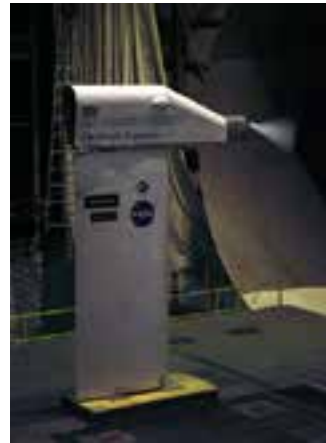
Testing of the Wright propellers was conducted using a NASA-developed thrust-torque balance, shown on the left, and the propeller-test-stand setup on the right. (ODU)
