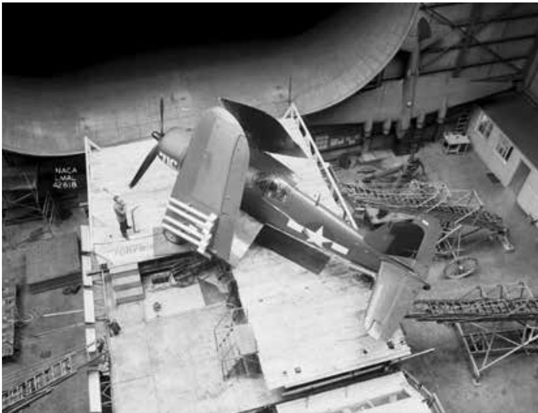
A Chance Vought F4U-1D Corsair prepares for wing-fold and wing-spread tests in 1945. Note the angle of yaw simulating a crosswind condition. Also of interest is the large Boeing B-15 model on the wall of the building. (NACA LMAL 42618)
