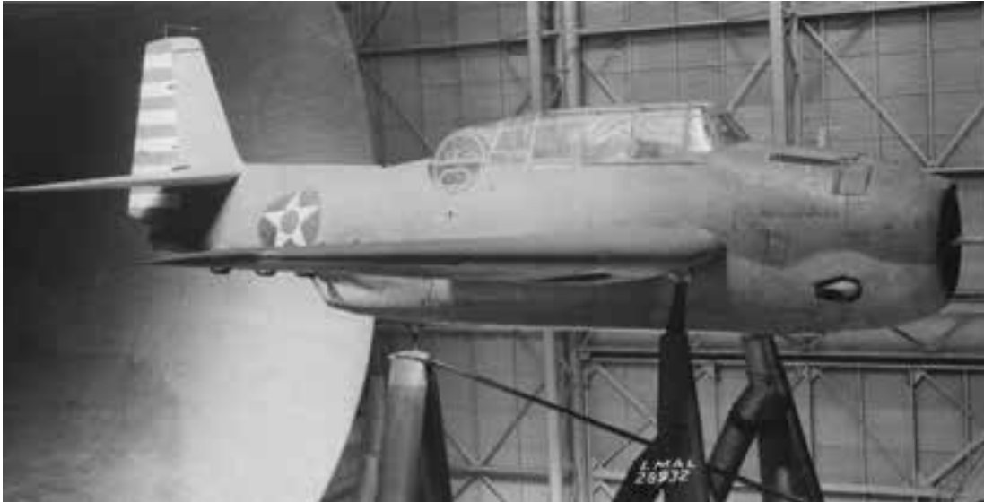
The second Grumman XTBF-1 prototype underwent drag cleanup testing in the Full-Scale Tunnel in 1942. (NACA LMAL 28932)
