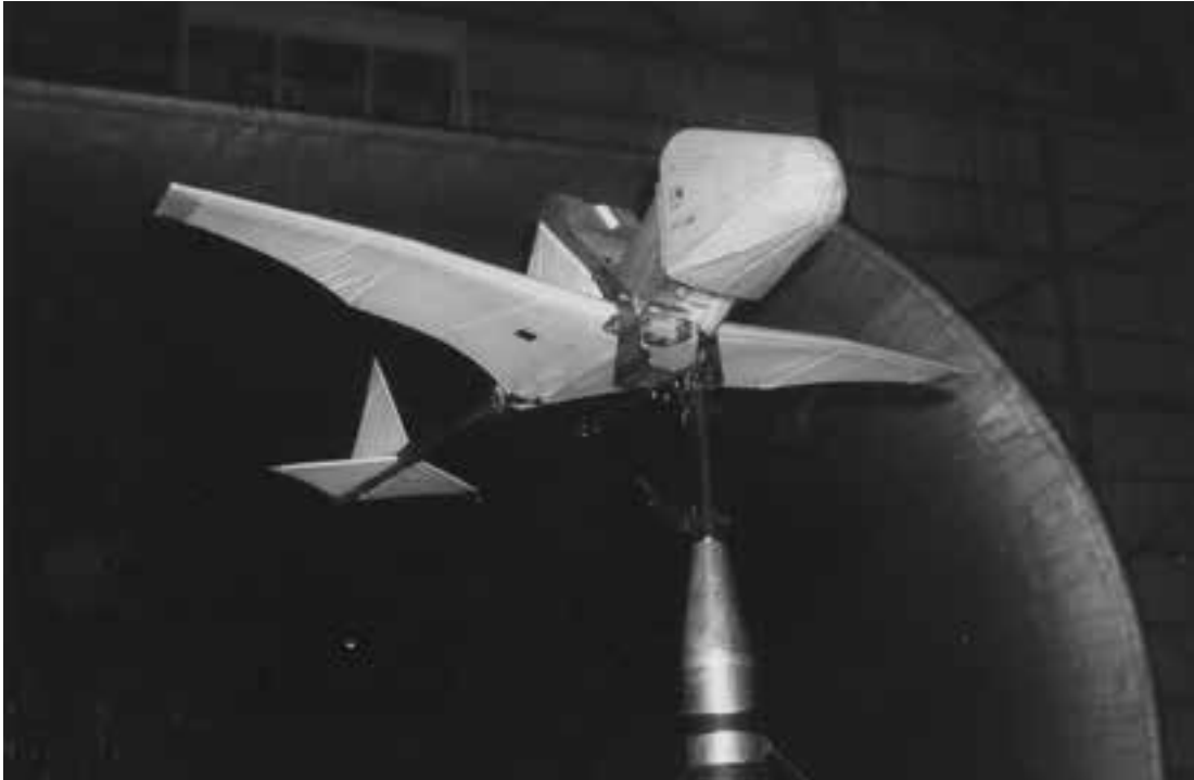
One of several configurations tested as part of an investigation of the aerodynamic characteristics of a flying ejection seat based on the application of the Princeton University sail-wing concept. (NASA L-70-4554)
