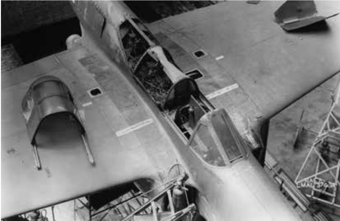
This photo of the cockpit area of the YP-59A was taken on April 26, 1944, and shows the cockpit damage sustained during an engine fire under powered conditions. The damage was repaired to an acceptable state and the tests continued until July. (NACA LMAL 37434)
