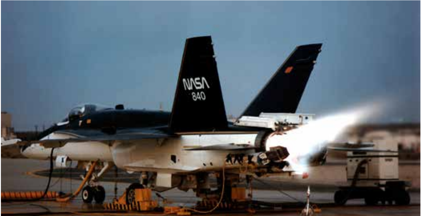
Spectacular engine test run for the HARV in 1994 with nose-up pitch control applied. (NASA EC 91-075-38)
