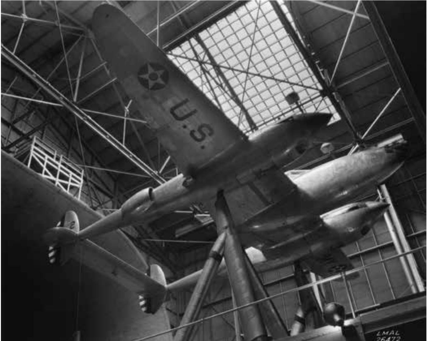
The third Lockheed YP-38 mounted for drag cleanup studies and predictions of the onset of compressibility effects in December 1941. The photo shows the aircraft in its service condition. (NACA LMAL 26472)
