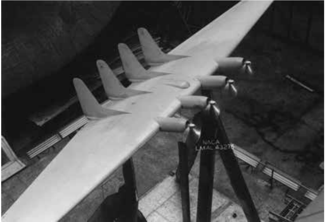
Model of the radical Kaiser Cargo Wing in powered tests (NACA LMAL 43276)
