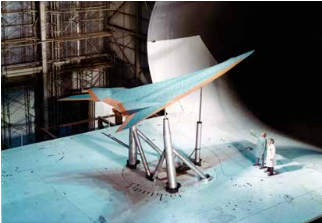
Technicians prepare the “platypus-nose” SCR model for testing in 1973. Note the two-dimensional thrust-vectoring engine nacelles. (NASA L-73-7547)
