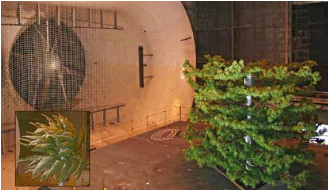
Tests of a cell-phone tower disguised as a tree were conducted in 2007 to determine aerodynamic loads. Note the protective net on the front of the exit cone. The inset shows another test configuration. (ODU)
