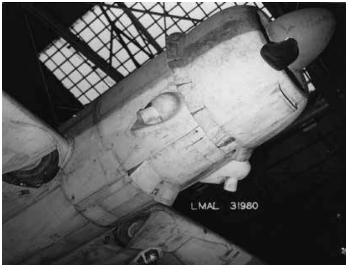
Shown are several major drag-contributing features of the SB2C-1, including the large-bore exhaust stacks and exposed wheel wells. (NACA LMAL 31980)
