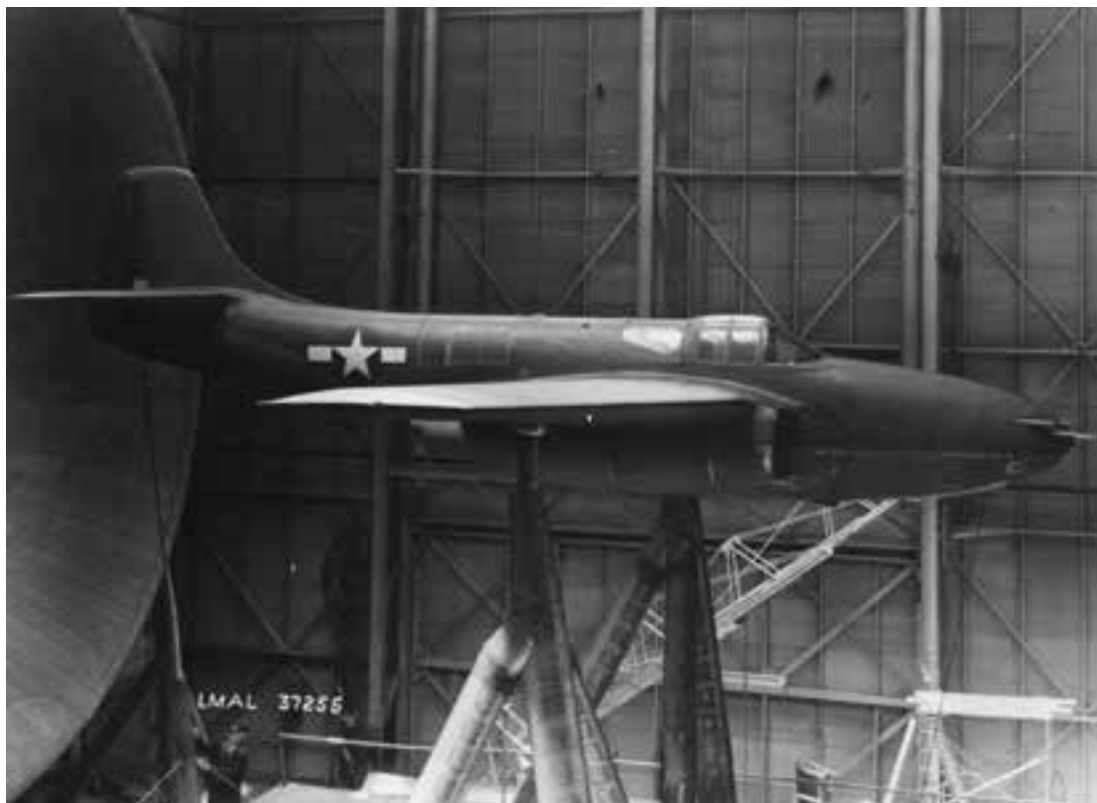
The YP-59A developmental prototype of America's first jet-powered military aircraft underwent extensive testing in the Full-Scale Tunnel in 1944. In this photograph, the aircraft is in the service condition. (NACA LMAL 37255)
