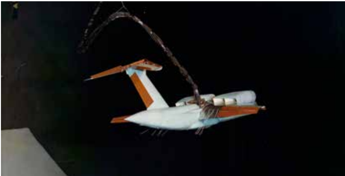
The powerful flow-turning capability of the upper-surface blowing concept is illustrated by wool tufts attached to the trailing-edge flap segments behind the upper-surface engines of this free-flight model in 1973. (NASA L-73-6289)
