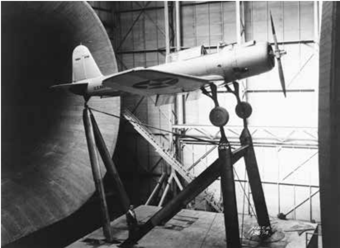
This Vought Vindicator, tested in the tunnel in late 1937, was the first production SB2U-1 aircraft. Its tunnel test program was abbreviated and consisted of measuring aerodynamic behavior at stall for correlation with flight tests. (NASA EL-2003-00283)
