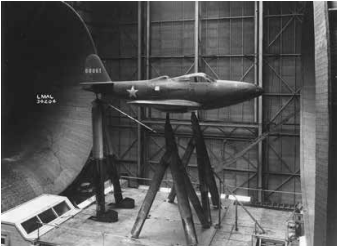
The Bell P-63A Kingcobra was the subject of a coordinated wind tunnel and flight investigation at Langley in 1943. In this photo, the aircraft is mounted in the Full-Scale Tunnel for drag cleanup tests. (NACA LMAL 34204)
