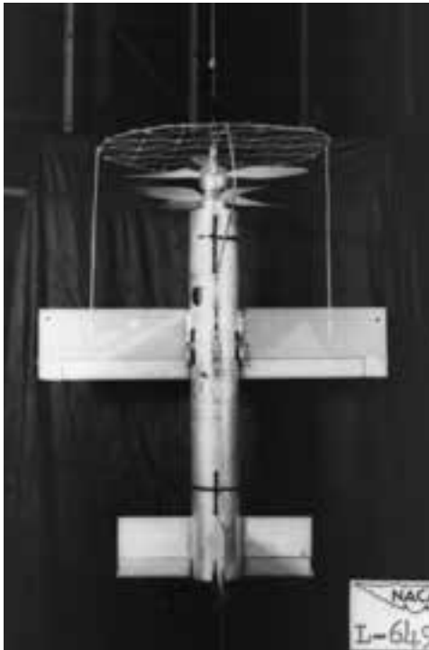
Left: This simple tail-sitter research model was the first VTOL free-flight model used in investigations of dynamic stability and controllability in 1949. (NASA EL-2001-00442). Right: The first free-flight model flown in the test section of the Full-Scale Tunnel was the Convair XFV-1 Pogo in 1952. Langley researchers Charles C. Smith (left) and Robert O. Schade (right) prepare the model for testing. Note the protective propeller shield installed to avoid inadvertent encounters with the flight cable. (NACA LAL-82885)
