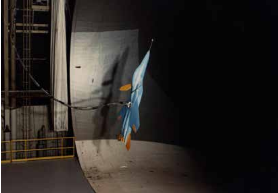
The F-15 STOL/MTD configuration was modified by the staff at the Full-Scale Tunnel to include vanes for yaw vectoring and demonstrate the general benefit of yaw vectoring for increased control at high angles of attack. The model was flown without vertical tails during some of the tests as shown here. (NASA L-88-01061)
