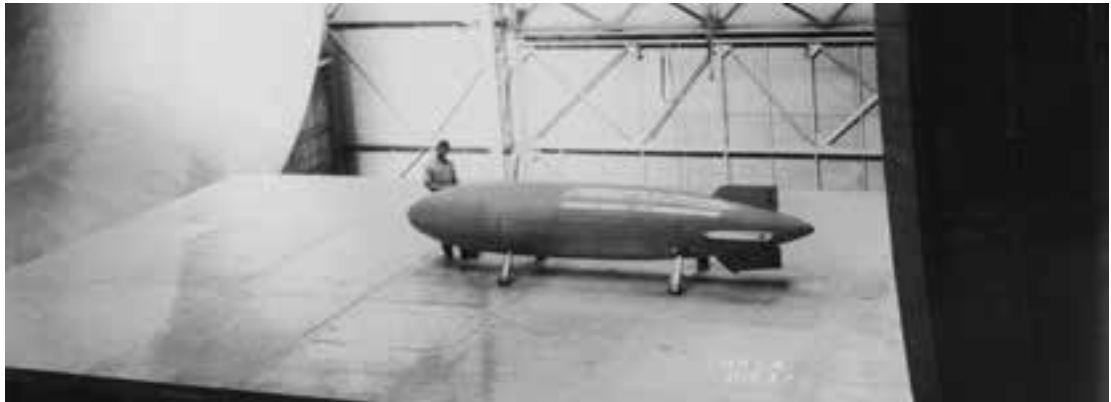
Navy-requested airship testing in the 1930s included assessments of ground-handling loads for the airship Akron (upper photo) and aerodynamic loads on the Lakehurst airship hangar (lower). The model of the Akron is being tested for rearward (flow from right to left) wind conditions. (NACA 11163 and NACA 11123)
