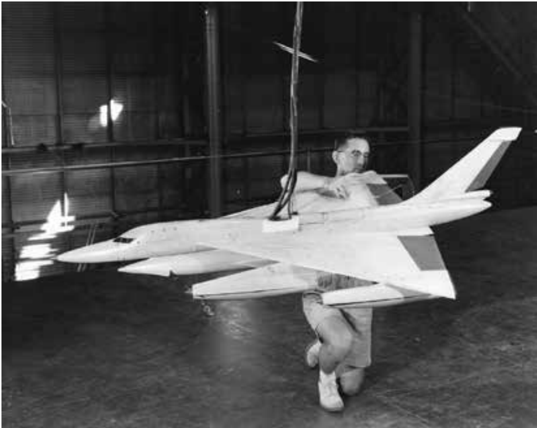
Free-flight tests of the Convair XB-58 bomber configuration provided information on the high-angle-of-attack dynamic stability control characteristics of the design. Technician Joe Block prepares the model for a flight test. (NACA L-96279)
