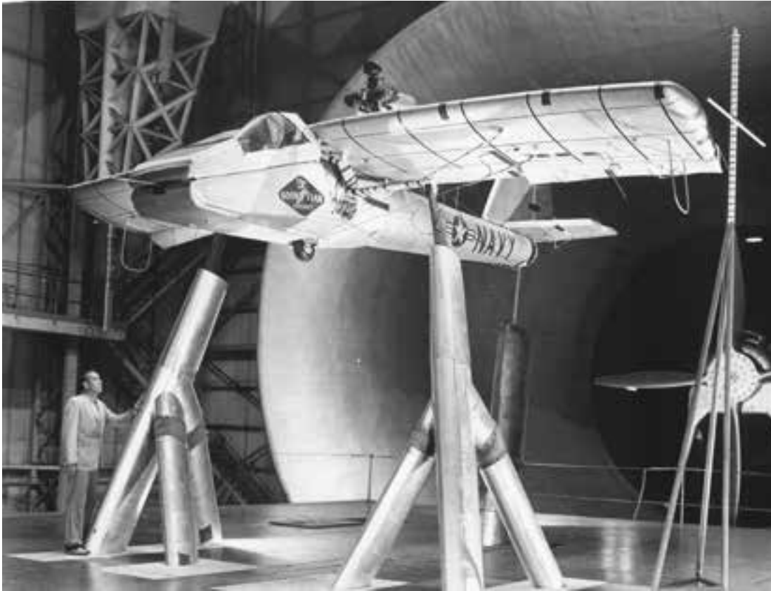
The Goodyear XAO-3 Inflatoplane had two separate test entries in the Full-Scale Tunnel. This photograph, taken during a 1957 investigation, shows the general arrangement of the inflatable aircraft. Note the wingtip ground-protection outriggers beneath the wingtips, the guy cables used to constrain the wing, and the vertical scale on the right used to measure wing deflections during tests. (NACA LAL-57-3413)
