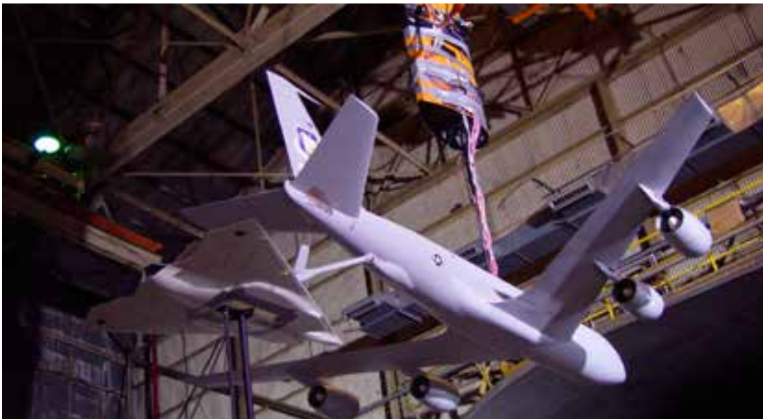
A model of a delta-wing uncrewed aerial vehicle is positioned to acquire aerodynamic data during a simulated air-to-air refueling mission behind a model of a KC-135R tanker. (BAR)
