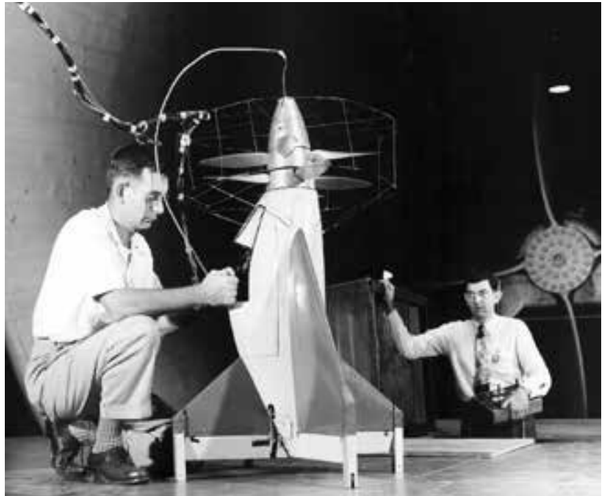
Left: This simple tail-sitter research model was the first VTOL free-flight model used in investigations of dynamic stability and controllability in 1949. (NASA EL-2001-00442). Right: The first free-flight model flown in the test section of the Full-Scale Tunnel was the Convair XFV-1 Pogo in 1952. Langley researchers Charles C. Smith (left) and Robert O. Schade (right) prepare the model for testing. Note the protective propeller shield installed to avoid inadvertent encounters with the flight cable. (NACA LAL-82885)
