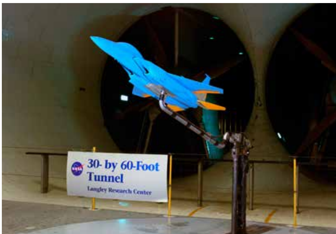
Langley updated its 23-year-old F-15 free-flight model to respond to an Air Force request for high-angle-of-attack testing in support of the F-15E Keep Eagle program. The photograph shows the 1/10-scale model during tests in the Full-Scale Tunnel in 1994 (NASA EL-1996-00064)
