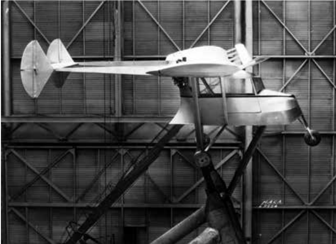
The Weick W-1 airplane incorporated several safety-enhancing concepts, including a tricycle landing gear. Note the fixed auxiliary airfoil ahead of the wing leading edge. (NACA 9554)
