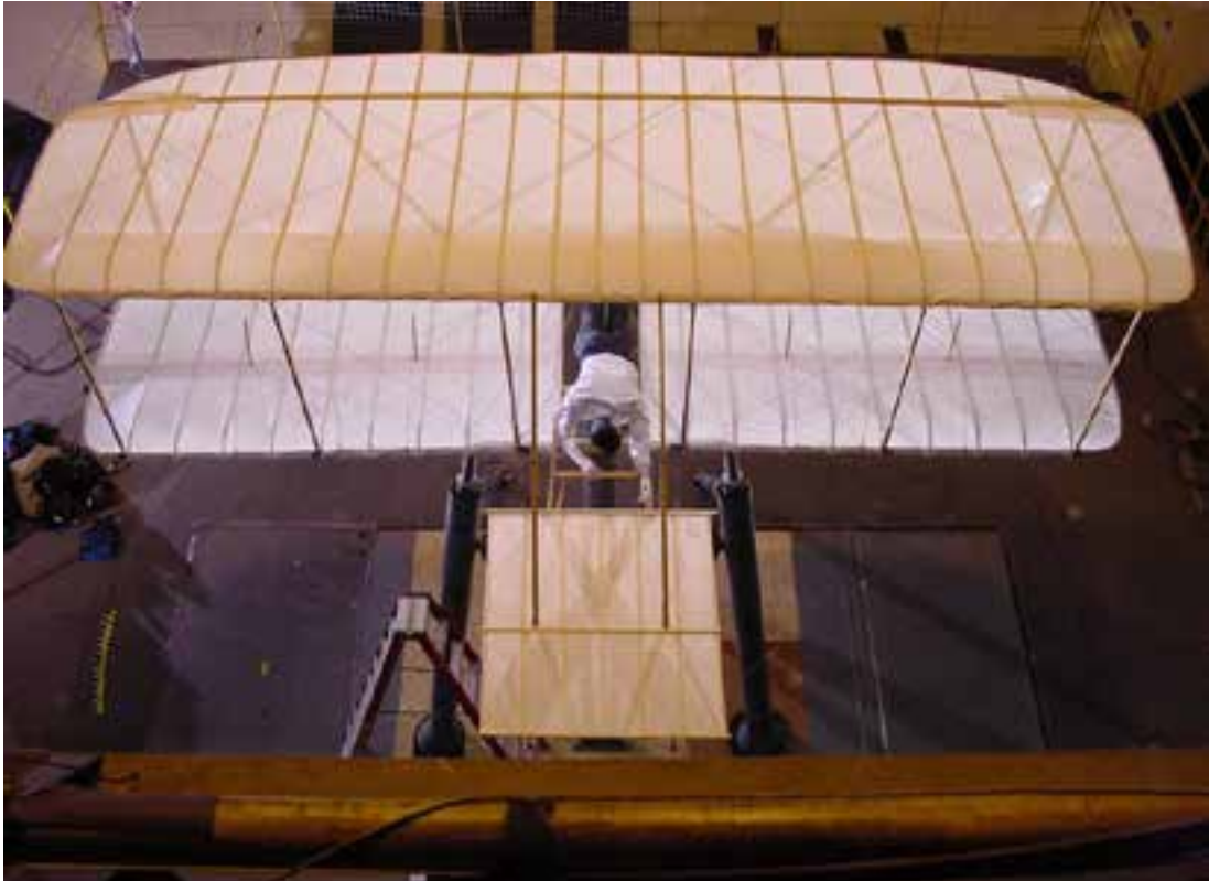
Overhead front view of the 1901 Wright glider test setup in the Full-Scale Tunnel. (ODU)
