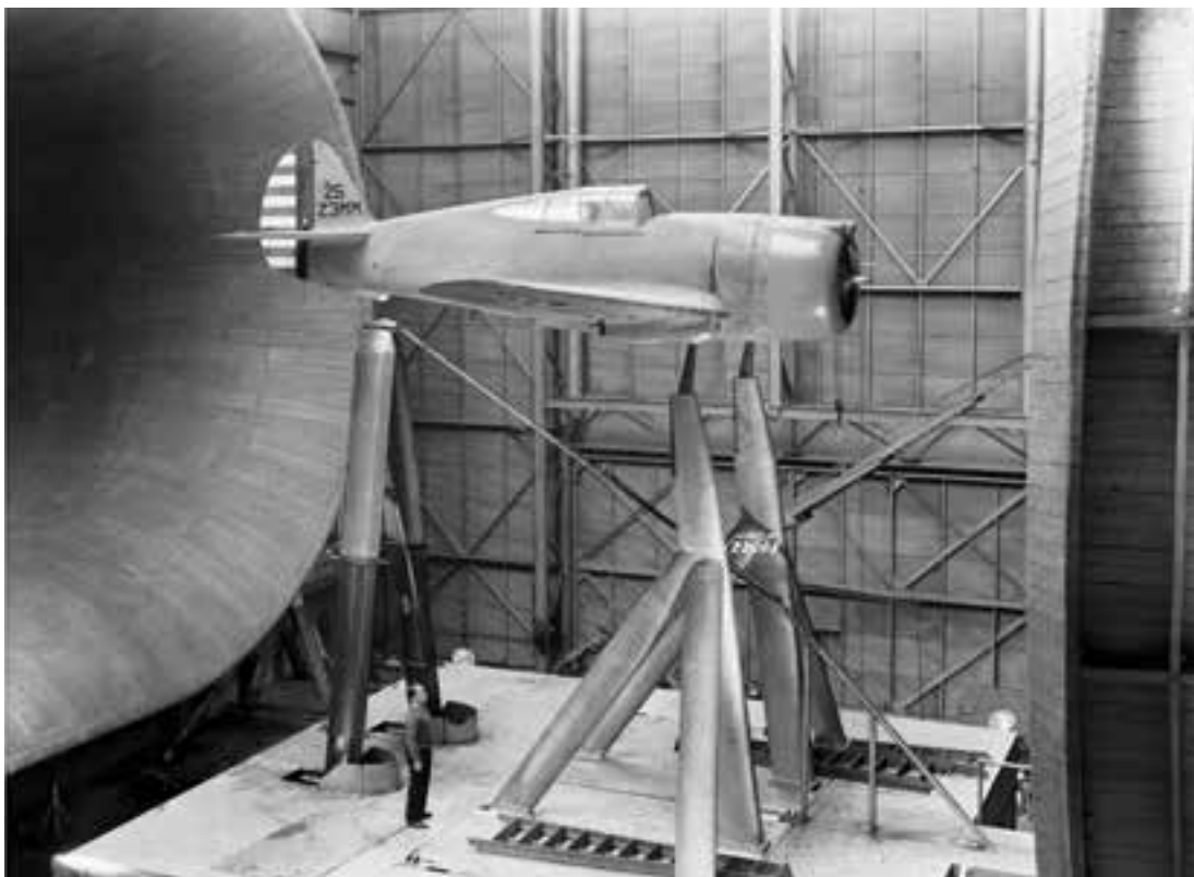
A Curtiss P-36C was tested in December 1940 as part of the NACA engine cowling program. (NACA 22128)
