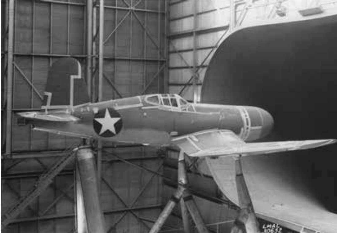
A Vought-Sikorsky F4U-1 Corsair was tested in the Full-Scale Tunnel and flown by Langley test pilots in December 1942. Here, the aircraft is in the faired and sealed condition for drag cleanup tests. (NACA LMAL 30652)
