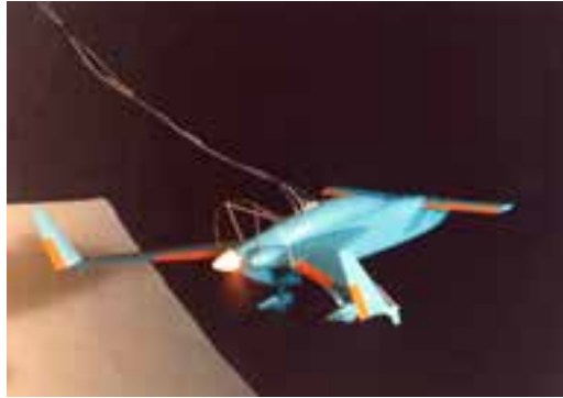
Free-flight model of the Rutan Varienze during stall-resistance testing in the Full-Scale Tunnel in 1980. Note the propeller-guard assembly used to protect the flight cable during the investigation. (NASA L-80-5673)
