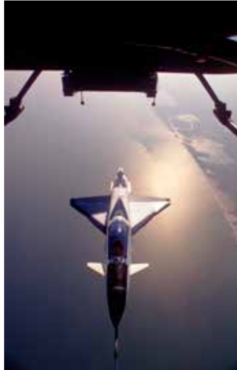
View of the tailless X-31 drop model as it falls away from the helicopter during a test at the NASA Wallops Flight Facility. The model was retrieved from a water landing following the use of an onboard recovery parachute. (NASA L-94-08995)
