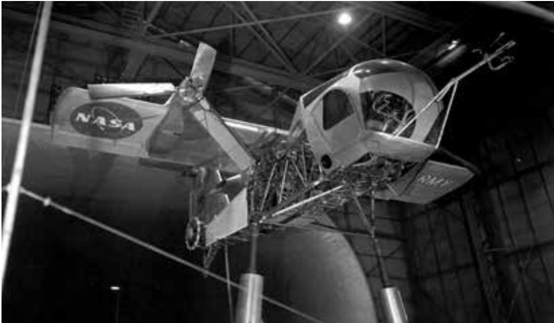
The full-scale VZ-2 tilt-wing airplane mounted for testing in the Full-Scale Tunnel in 1961. The original configuration was prone to wing stall and exhibited uncontrollable lateral directional motions during partial-power descending flight. Tests in the Full-Scale Tunnel demonstrated the effectiveness of wing modifications to minimize the problem. (NASA L-61-1767)
