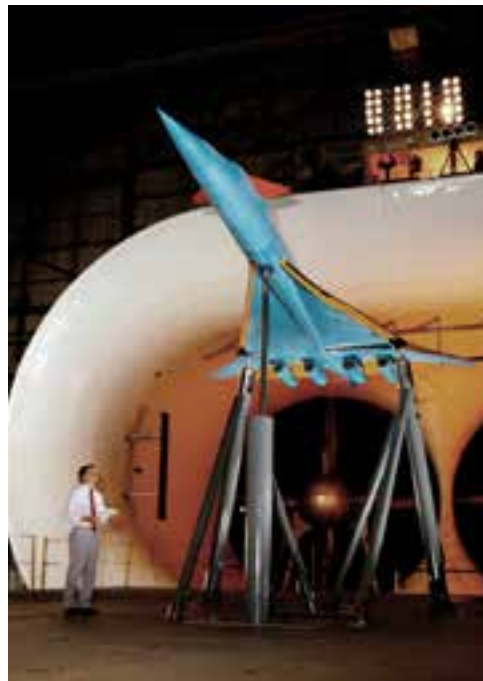
Researcher Dave Hahne poses in 1992 with a large-scale model of a Mach 2.2 supersonic transport concept designed by the Douglas Aircraft Company. The test produced a large database of aerodynamic data for low-speed performance, stability, and control, as well as pressures on the wing leading edge. The primary goal of the test was to compare the aerodynamic performance of a 20-year-old constant-chord leading-edge flap with that obtained with a tapered flap designed by computational methods. (NASA L92-12858)
