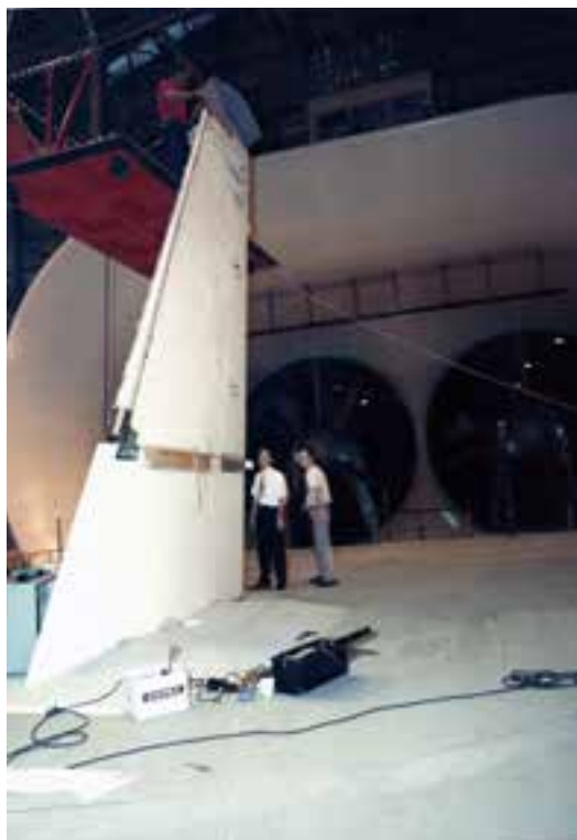
A full-scale semispan of an EA-6B aircraft was tested in the Full-Scale Tunnel in 1991 to measure detailed aerodynamic data for a modification to use the wingtip speed-brake surfaces as ailerons. The conventional EA-6B aircraft used split upper and lower surfaces to control airspeed during carrier approaches. In the Full-Scale Tunnel studies, the surfaces were coupled to permit deflections as a single conventional aileron for improved controllability at high angles of attack. (NASA L-91-11228)
