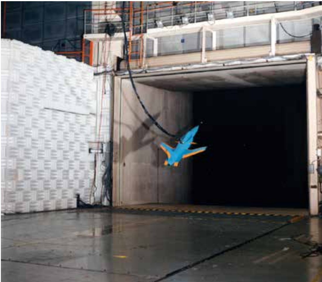
An existing free-flight model of the X-29 forward-swept wing aircraft was used to evaluate the feasibility of conducting free-flight tests in the Langley 14- by 22-Foot Tunnel. The photograph shows the model in flight in the open-throat test section. The remote flightcrew was housed in a temporary enclosure to the right of the picture. (NASA L-94-03947)
