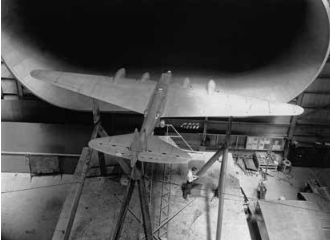
The huge 1/4-scale model of the XB-15 was used for assessments of the aerodynamic characteristics of the airplane as well as for generic studies of engine installations by the NACA. In this 1936 photograph, the model is mounted for tests of the configuration in yaw. (NACA 12088)
