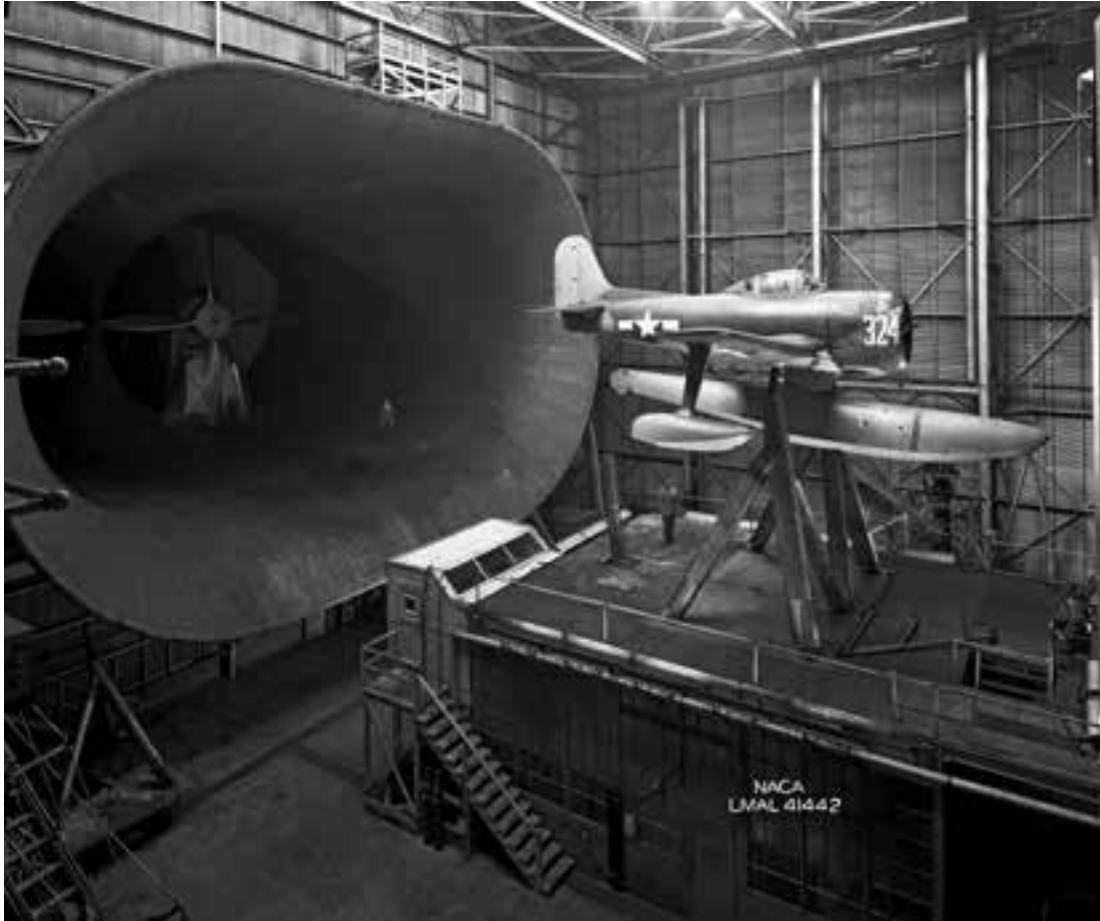
Curtiss SC-1 Seahawk scout mounted for drag cleanup, stability and control, and cooling tests in December 1944. (NACA LMAL 41442)
