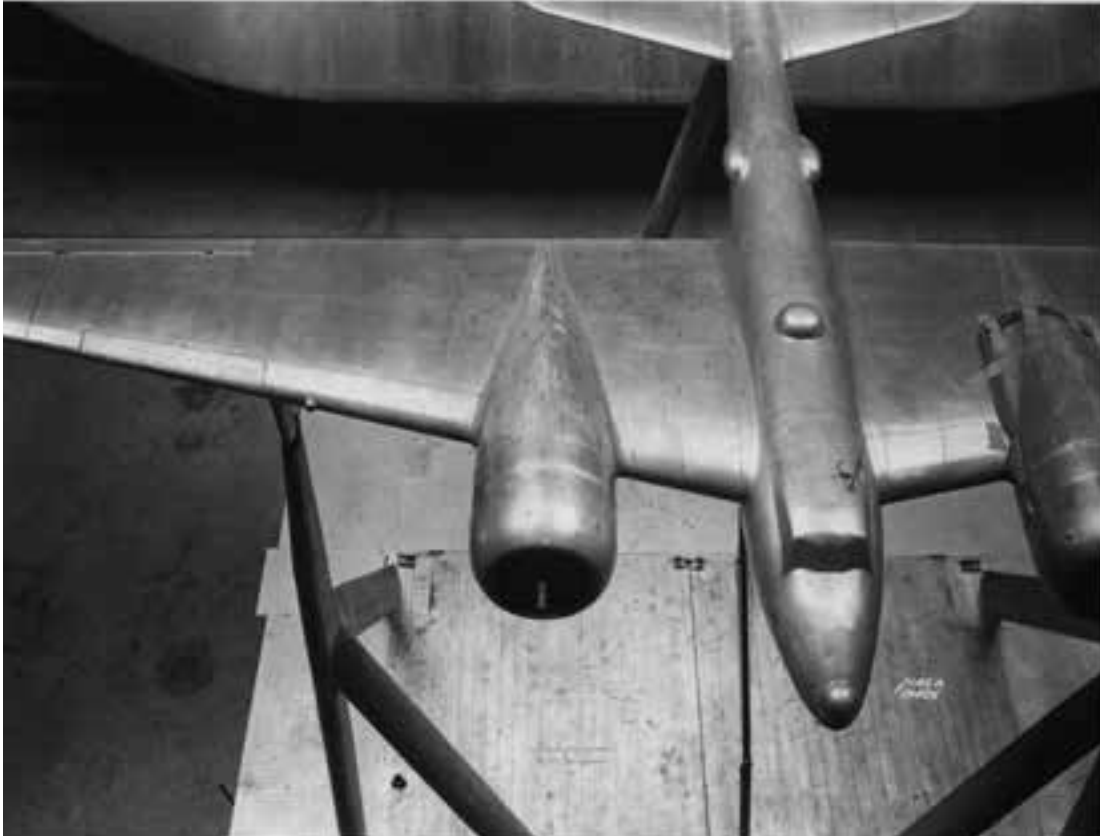
The XBLR-1 model was loaned by the Army to the NACA and served as a test bed for many projects. Here the model has been modified as a twin-engine configuration with air-cooled engines in February 1940. (NACA 19406)
