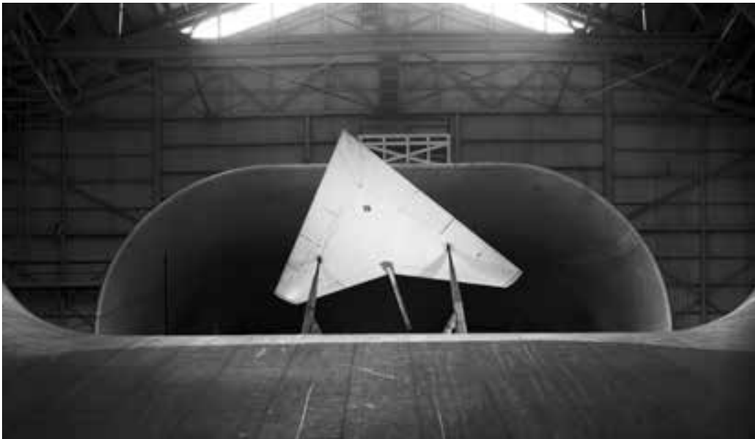
This large-scale arrow wing model with clipped wingtips was one of a series of supersonic wings tested in the Full-Scale Tunnel. (NACA LMAL 57083)
