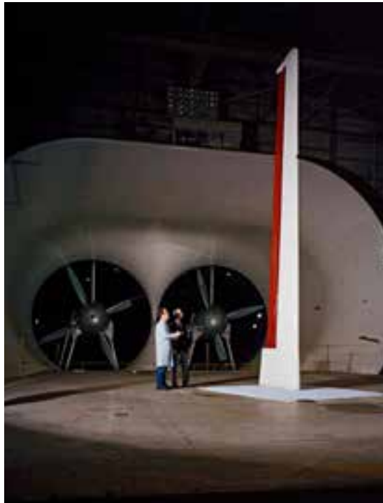
Technician Dave Brooks (left) and researcher Frank Jordan (right) discuss the test plan for a 24-foot-long outer blade of a windmill in 1984. The project was sponsored by the Wind Energy Project Office at the NASA Lewis Research Center with the objective of investigating the effects of ailerons on the controllability of large windmill blades. (NASA L-02783)
