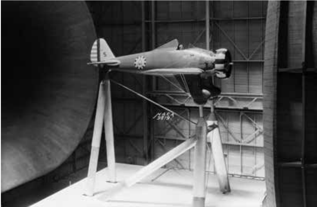
The objective of tests of the Boeing P-26 aircraft in the Full-Scale Tunnel in May 1934 was to define the benefits of wing flaps on reducing the landing speed to enhance safety of flight. (NASA EL-1999-00623)
