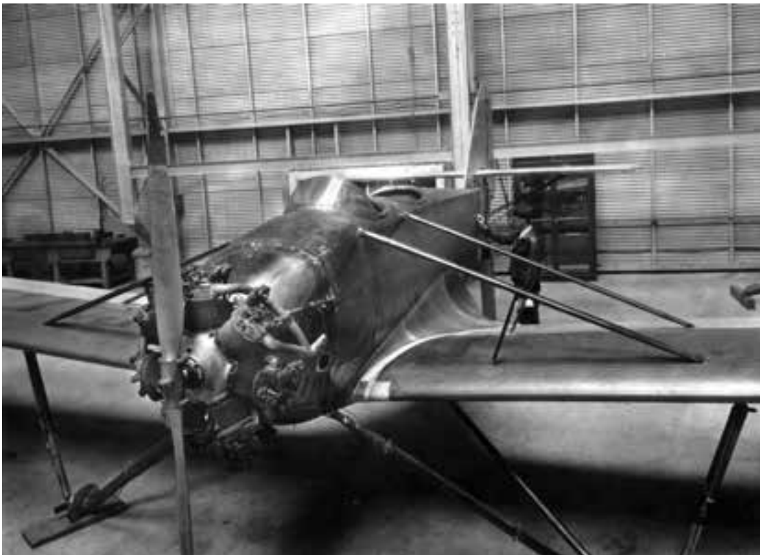
This front view of the Doodlebug shows the aircraft without an engine cowling and with one of several wing-root fillets conceived by the Langley staff. (NACA 8145)
