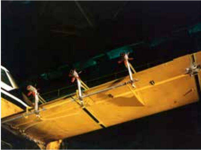
Near-field spray characteristics were determined in the Full-Scale Tunnel by spraying water from the airplane's dispersal system. The spray-bar arrangement is shown on the left, and dispersal testing showing the water spray is shown on the right. (NASA L-78-4148 and NASA L-78-4061)
