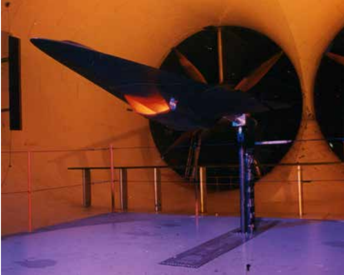
The LoFLYTE configuration undergoes static force tests in the Full-Scale Tunnel in 1995. (NASA L-95-04052)
