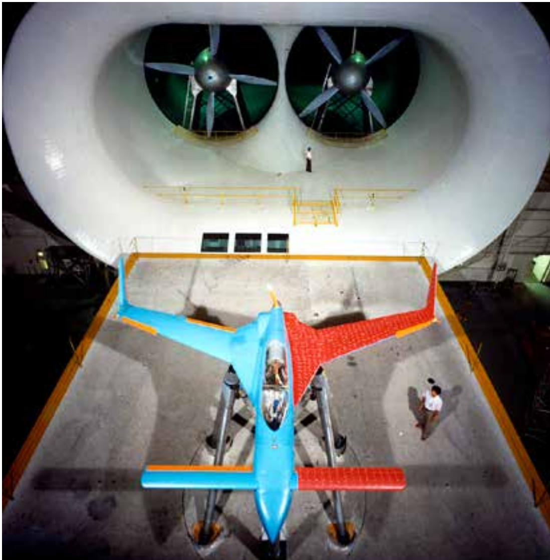
Researcher Long Yip inspects the full-scale model of the Varienze during tests in 1981. The left side of the model has been painted to enhance flow visualization, and wool tufts were affixed to the wing upper surface for flow-visualization tests. Note the discontinuous leading-edge droop segments added to the wing for the study. (NASA L-81-7333)
