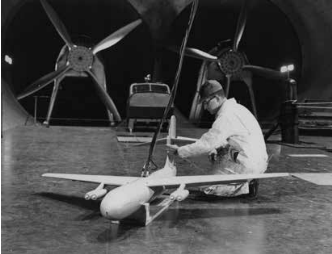
Technician Joe Block prepares the first Langley EBF free-flight model for tests in the Full-Scale Tunnel in 1956. At the time, John Campbell's group was still located at the 12-Foot Free-Flight Tunnel. (NACA LAL 96823)
