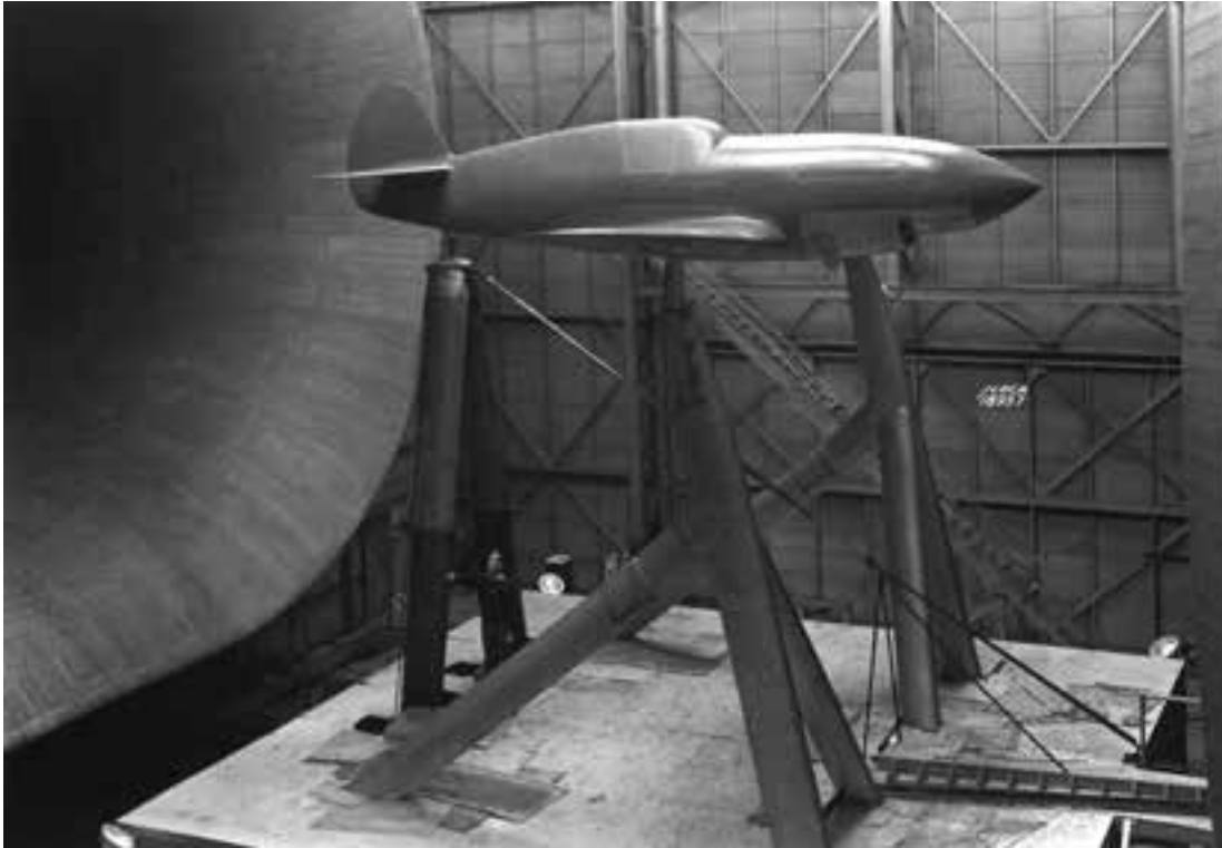
The full-scale model of the Curtiss XP-46 mounted for tests in November 1939. The model was fabricated from wood with an external finish of glazing clay polished to a mirror-like smoothness. (NACA 18957)
