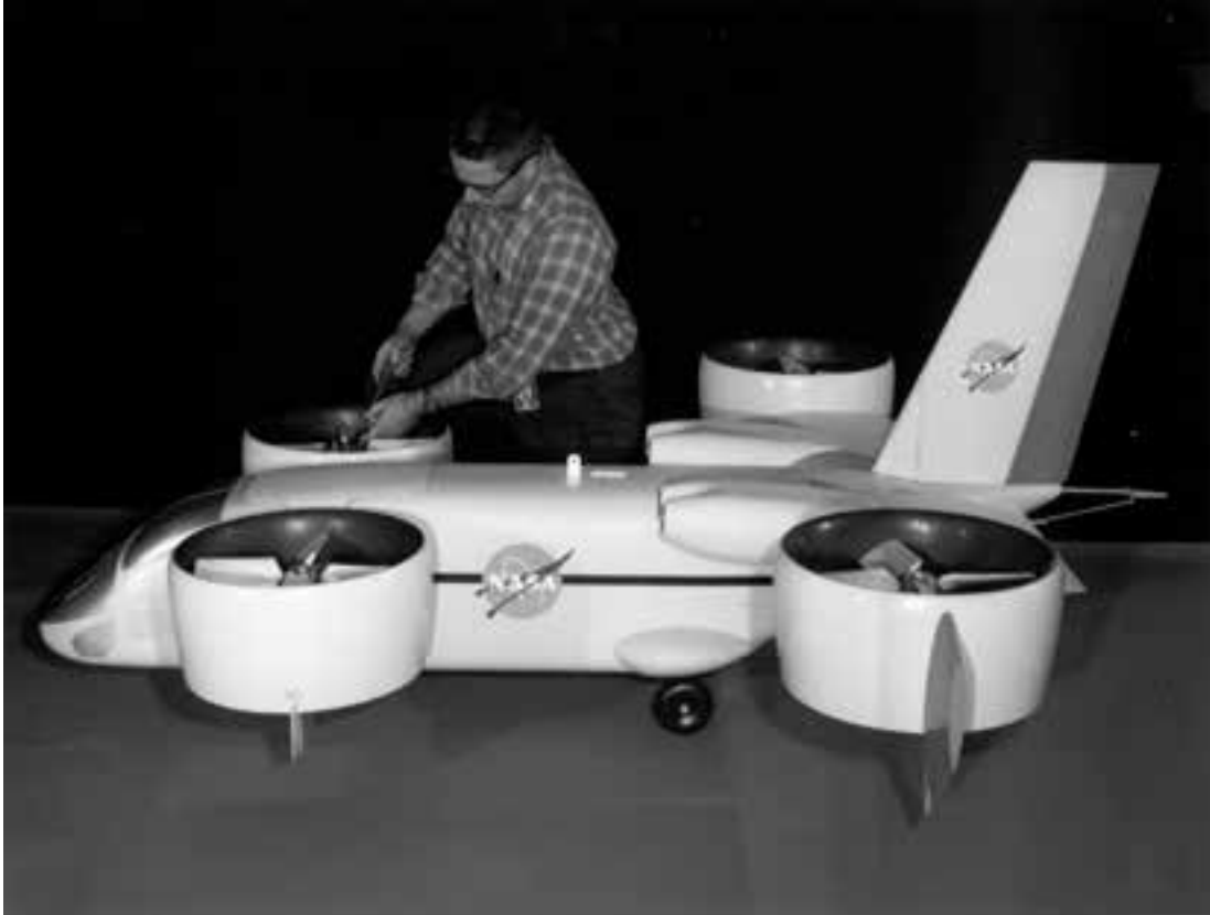
Researcher Bill Newsom poses in 1963 with a free-flight model of the Bell X-22A tilt-duct V/STOL configuration prior to free-flight testing in the Full-Scale Tunnel. (NASA L-63-10043)
