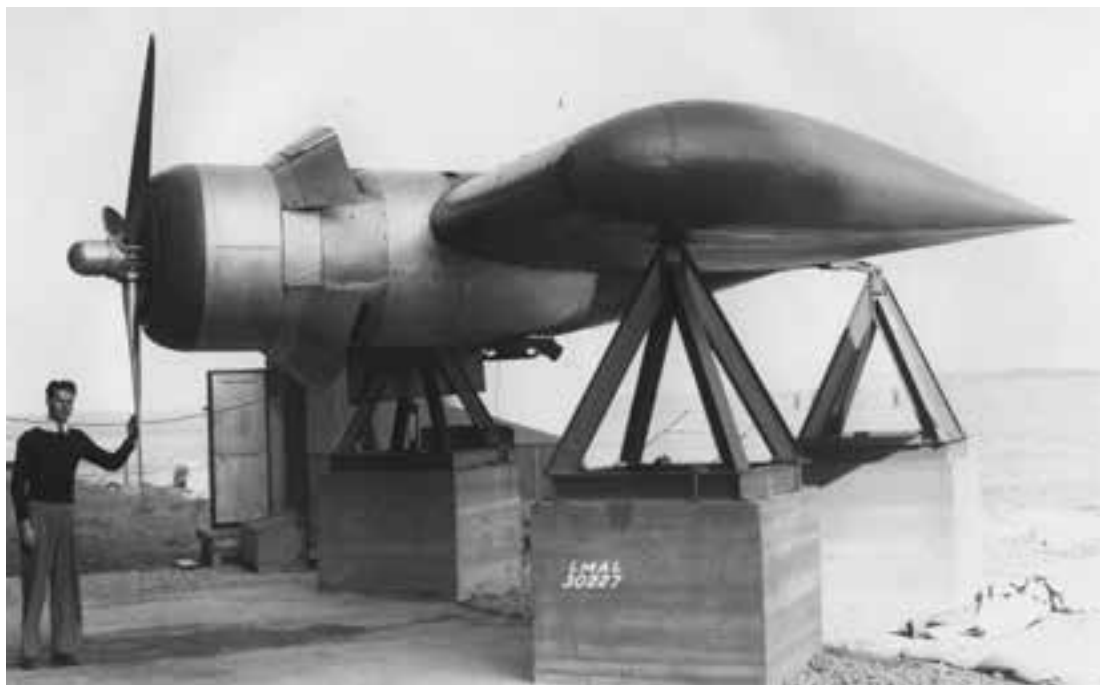
The staff of the Full-Scale Tunnel responded to an urgent Army request to mitigate B-24 engine-heating problems by testing hardware outside the tunnel on the bank of the Back River. Langley engineer Bruce Esterbrook poses with the test setup. Note the oversized nacelle cowl flaps and the instrumentation read-out room behind the test article. (NACA LMAL 30227)
