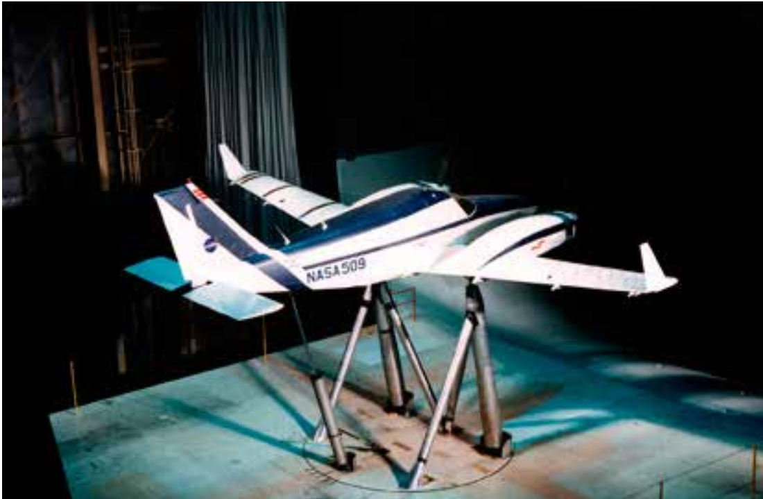
The Advanced Technology Light Twin-Engine research aircraft mounted for tests in the Full-Scale tunnel in 1977. (NASA L-77-2768)
