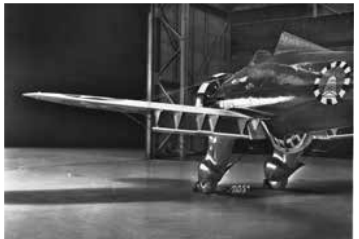
Shown on the ground floor of the Full-Scale Tunnel, the P-26 exhibits a split-flap concept evaluated during the test program. Rear view shows the wing flaps as well as the curved-flap segment beneath the fuselage. (NACA 9923 and NACA 9922)
