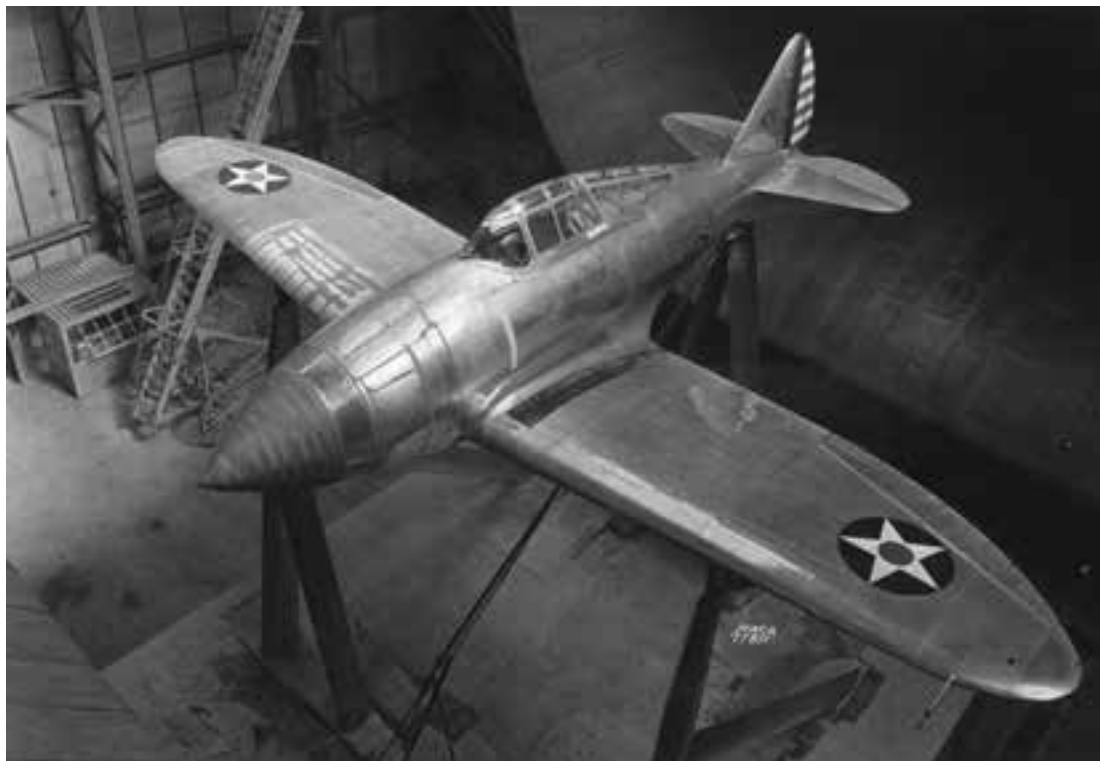
The Seversky XP-41 began a drag cleanup test program in the Full-Scale Tunnel in June 1939. In this photograph, the airplane is in the “sealed and faired” condition and at a cruise attitude. (NACA 17822)
