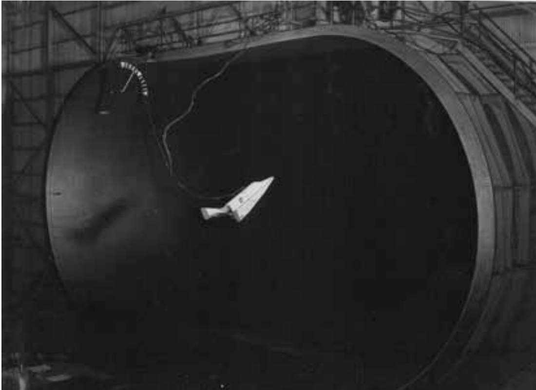
The Full-Scale Tunnel was used for extensive free-flight and force testing of the U.S. Air Force Dyna-Soar reentry glider in 1960. (NASA L-60-8494)
