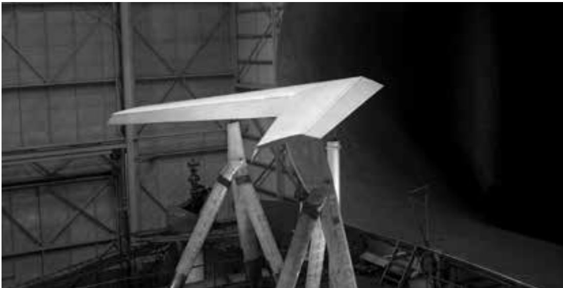
High-lift tests of a 45° swept wing with symmetrical circular-arc sections evaluated the effect of leading- and trailing-edge flaps in 1946. (NACA LMAL 50361)
