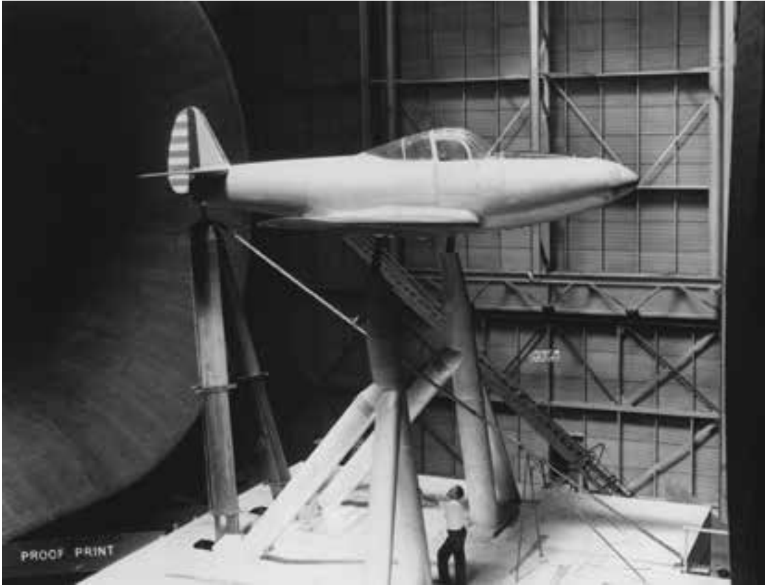
The Bell XP-39 test in 1939 was the most controversial test ever conducted in the tunnel. The upper photo shows the airplane in the faired condition without the oil-cooler intake on the right rear fuselage. The bottom photo shows the airplane with the canopy removed. The person on the ground board is Abe Silverstein. (NACA 18281 and NACA 18212)
