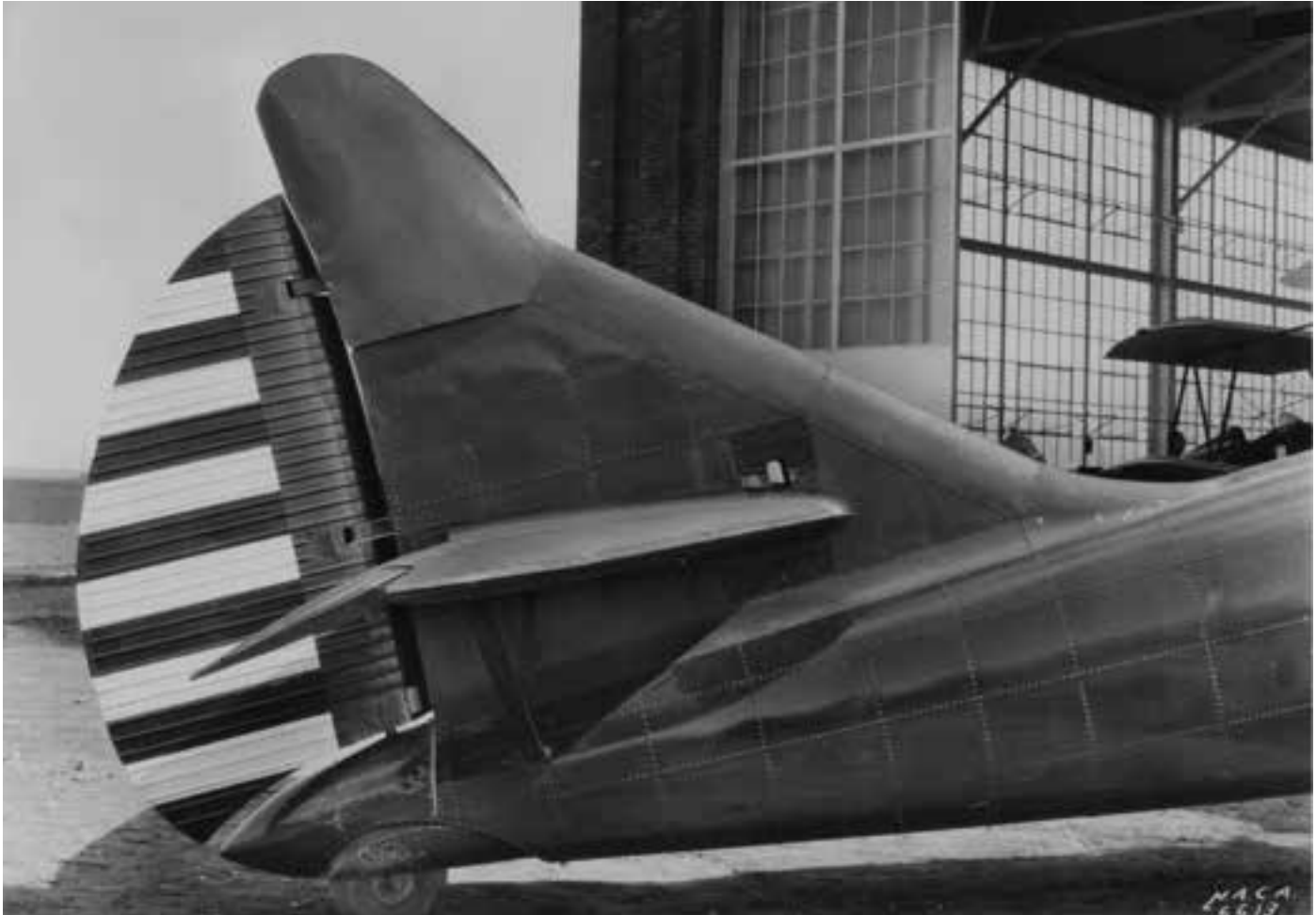
A close-up view of the radical vertical-tail extension conceived in the Full-Scale Tunnel tests for the YO-31A. The aircraft is parked following the wind tunnel tests near the entrance doors of the recently completed NACA flight hangar in 1932. (NACA 6613)
