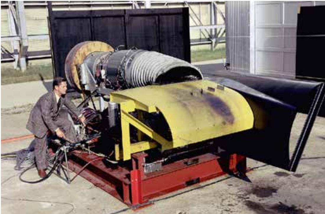
Engineer Jim Hassell poses with a large-scale component model of the YC-14 USB installation at the outdoor test site of the Full-Scale Tunnel. Note the vortex generators placed behind the engine to enhance turning of the flow. (NASA L-73-7729)
