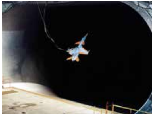
Mark Croom inspects a three-surface version of an F/A-18 free-flight model in 1982. In addition to forebody canards, the model was equipped with vanes to provide thrust vectoring for yaw control at high angles of attack. The three-surface F/A-18 research model flies at high angles of attack in the Full-Scale Tunnel in 1983. (NASA L-82-7534 and NASA L-83-4692)
