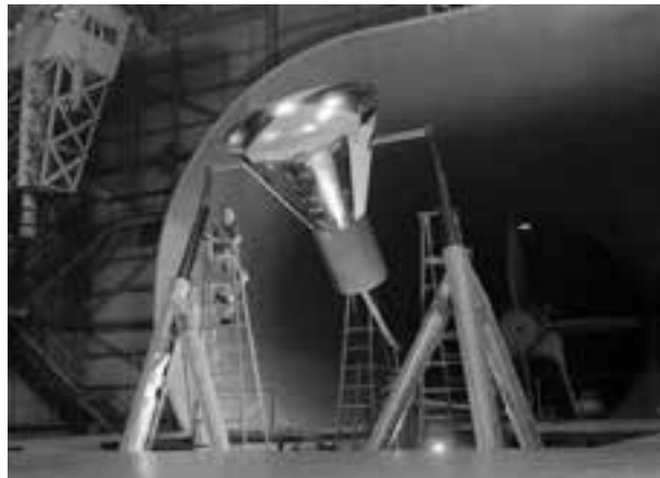
A full-scale model of the Mercury capsule is inspected by Clarence D. “Don” Cone during tests in January 1959. (NASA EL-1996-00094)
