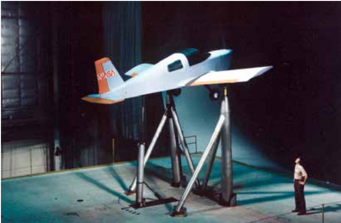
A full-scale model of a low-wing airplane used in the Langley stall/spin program was used for 1979 evaluations of a tail-spoiler concept for limiting angle of attack. (NASA L-79-07120)
