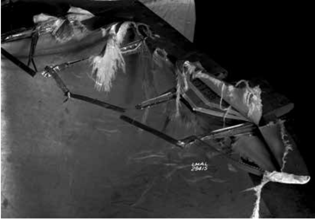
Photograph of the remains of a P-47B rudder after high-speed tests in the Langley 8-Foot High-Speed Tunnel resulted in structural failure at 460 mph. The top of the fabric-covered rudder (bottom right) failed, the fabric ripped, and the trailing edge went down the tunnel. The trailing edge segments (left) are held together with wire for the photograph. The failure occurred in less than 5 seconds. (NACA 29415)
