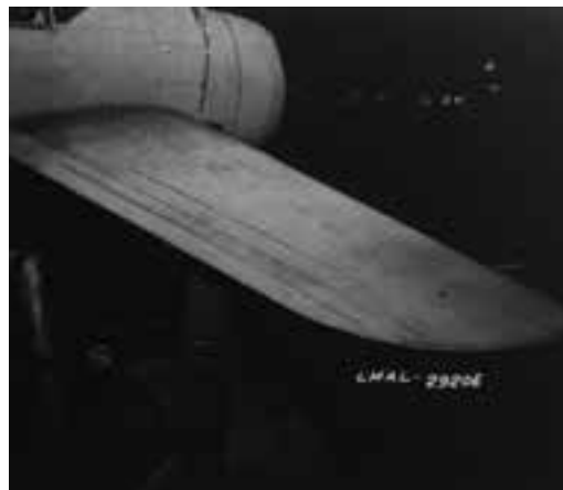
Views of the F2A-2 in the Full-Scale Tunnel with various deflections of the full-span slotted flap. Top photos show the flap deflected (left) and undeflected (right), while lower views show slot-lip ailerons deflected (left) and undeflected (right). (NACA 29206 to NACA 29209)
