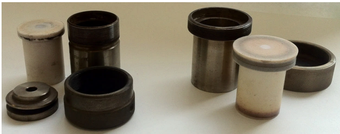
Figure 2.1 Example of autoclaves used in this study. The Parr type, 23 mL autoclave ( left ) and a 40 mL autoclave made in-house ( right ).
