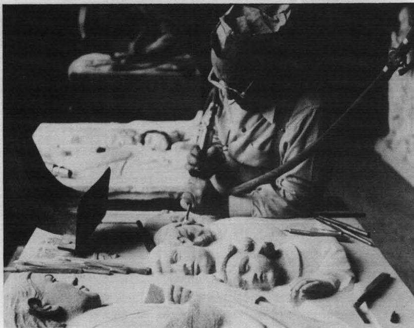
FIGURE 27. Carver sculpturing a bas-relief with a fine pneumatic chisel. Note variety of tool bits used. (1955.)
