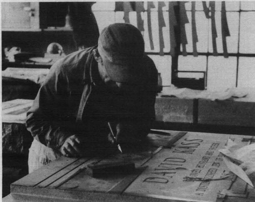
FIGURE 28. Cutting design through sheet of rubber cemented to stone prior to sandblasting. (1955.)
