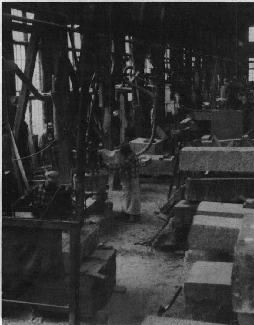
FIGURE 15. General view inside of typical stone shed showing local exhaust at each work station. (1955.)
