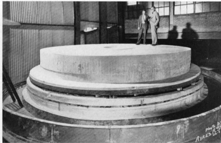
4. Out of the annealer, the mold which formed ribbed structure was removed before shipment.
