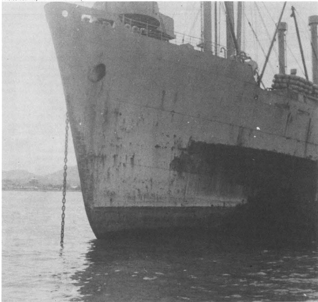
A port profile of Sommelsdijk showing some of the above waterline damage.
