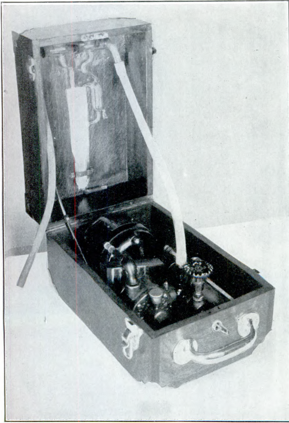
FIGURE 1.—ELECTRICALLY DRIVEN SUCTION APPARATUS FOR IMPINGER.
